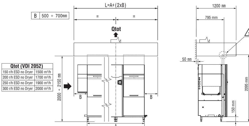
All exhaust hoods must be dimensioned and installed according to local regulations and industry standards which may differ from the recommendations herein suggested. Electrolux Professional is not liable for any failure in complying with local design standards.
